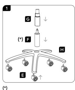
EN Remove the protective cover located at the top of the elevator before installation.
